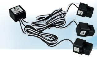
**CT clamp:** Current Transformer, an electrical device for non-contact measurement of current in a conductor. CT clamps are intended to be installed on the current-carrying live conductors ahead of the MCB. They monitor the total installation power (e.g., of an entire house or parking lot) and relay the values to the charger unit, which can then regulate its output power to prevent the MCB from tripping.
